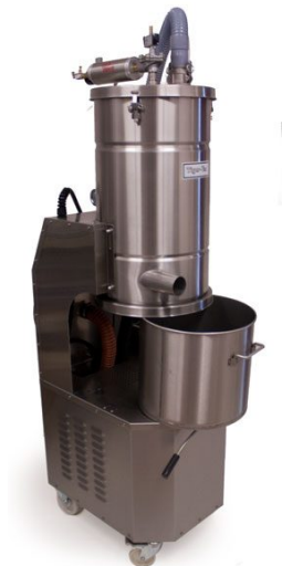
Tiger-Vac CD-2600 with the 36 litre recovery tank rolled out for emptying
